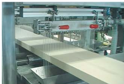
Separate application for resin and hardener
