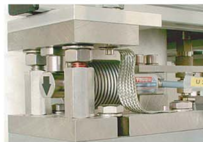
Weighing cell at the mixing unit
