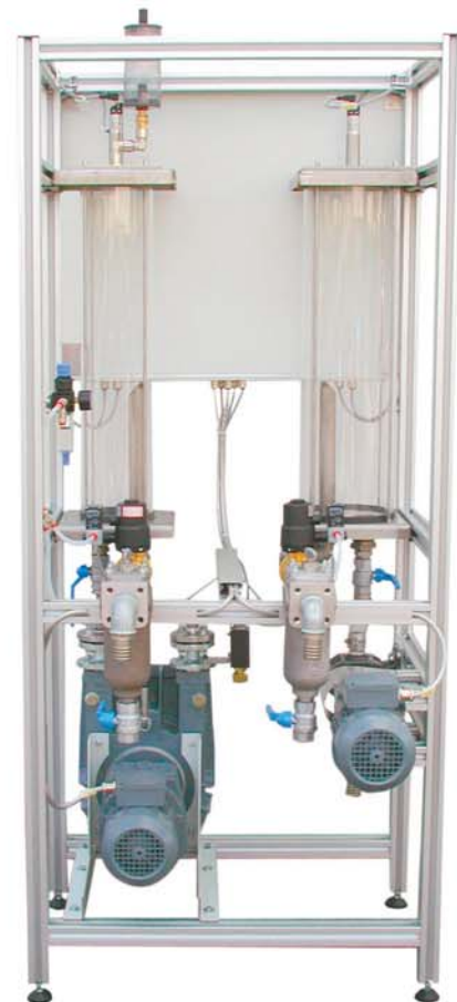
EPI-machine with intermediate storage vessels and dosing monitoring by sonar sensors
