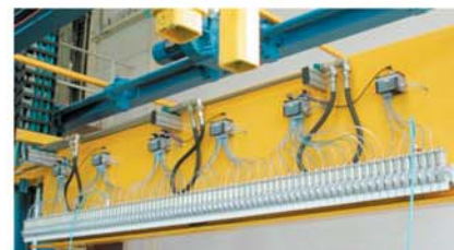
Application head: pouring width 3.000 mm
